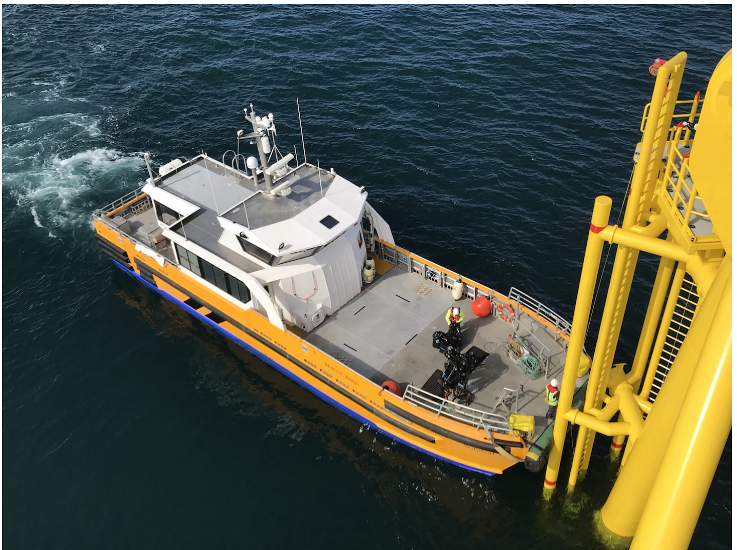
Image of a CTV making a transfer of a technician to an offshore wind turbine
